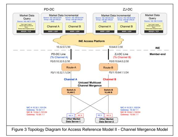
As shown in Figure 3, the shared tunnel model will use the existing network architecture, we simply need to enable the multicast function within this architecture, so the existing network is compatible with unicast/multicast transmission. This model is recommended to members who already deployed a a non-HSRP+NAT mode, below are the details of the deployment:
