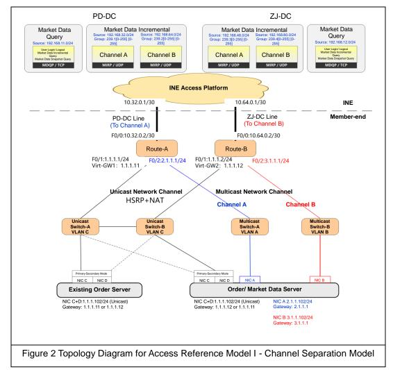
As shown in figure 2, the "Separated Tunnel Model reduces the impact on members' unicast networks. This model applies a new multicast network in parallel without affecting the existing unicast network architectures. This model is recommended to members who already deployed the HSRP+NAT mode, below are the details of the deployment:
